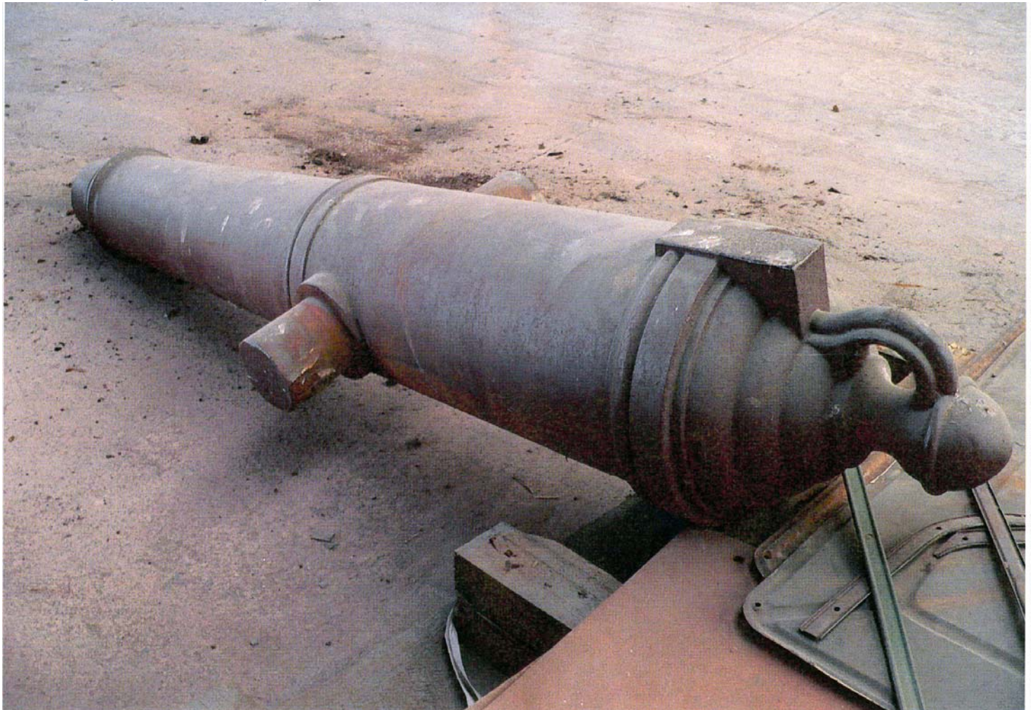
Above cannon is possibly Carron design c1840 -50 very well made much lighter in weight and probably made of the much stronger malleable cast iron but has no markings. The trunnions are concentric with the bore
