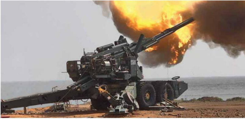
The advanced towed artillery gun system (ATAGS) is a towed 155 mm/52 calibre howitzer designed and developed in India
